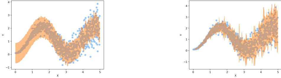
Figure 1.5: Comparison of interval lengths for absolute residuals V(x, y) = |y - \hat{\mu}(x)| (left panel) and rescaled residuals V(x, y) = \frac{|y - \hat{\mu}(x)|}{\hat{\sigma}(x)} (right panel).
