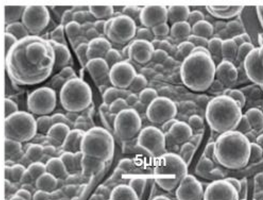
Figure 4.7: SEM image (30° tilt) of the electrodeposited catalyst after 30 C/cm^2 were passed in 0.1 M KPi electrolyte (at pH 7.0) which contains 0.5 mM of Co^{2+} .
