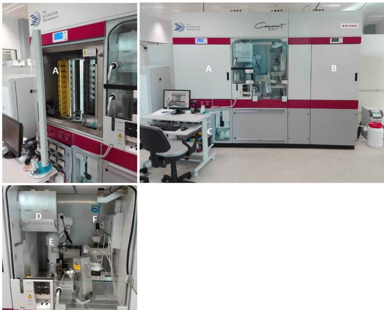
Figure S2: Overview of the Compact Select platform. (A) Flask carousel incubator, (B) Plate incubator, (C) Media pumps, (D) Decappers, (E) Robot arm, (F) Pipette head.
