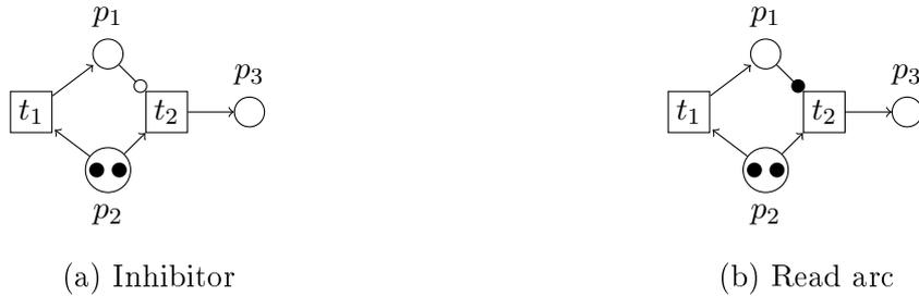
Figure 2.2: P/T nets with inhibitor and read arcs
