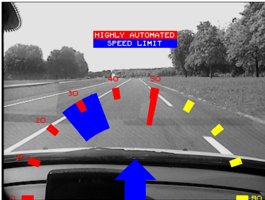
Figure 4.8: Scenarios *Following a human target speed* and *Approaching a speed limit* on LIVIC Legal Safety Vehicle: HMI at  $t = 21$  s. Subject speed is 50 km/h, matching human target speed. Current speed limit is 90 km/h. A future speed limit of 30 km/h has been detected
