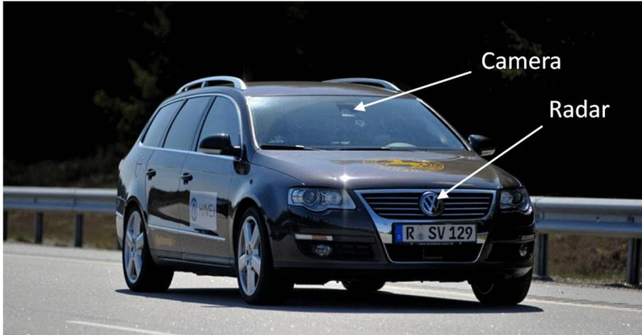
Figure 4.28: HAVEit Architecture Migration Vehicle with camera for lane perception and radar for object perception
