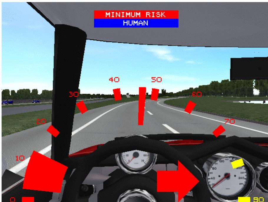
Figure 4.21: Scenarios *Decreasing or increasing automation mode to DA, SA, HA, FA and MRM* on LIVIC Legal Safety Simulator. Subject speed is 47 km/h, human target speed 70 km/h and speed limit 90 km/h. The subject has started an MRM, it decelerates and performs multiple lane changes towards the emergency lane
