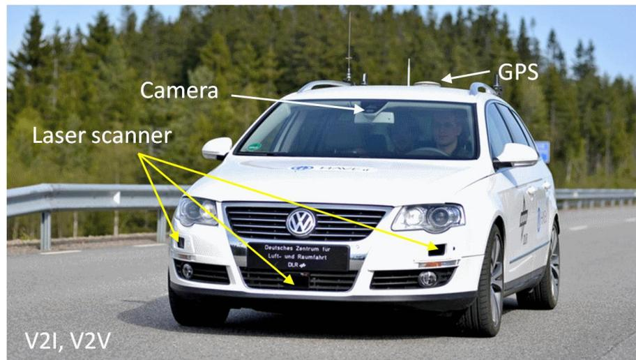
Figure 4.25: HAVEit Joint System Vehicle with camera for lane perception and LIDAR for object perception. The GPS, V2I and V2V communication are used for the detection of stops, speed limits and priority vehicles
