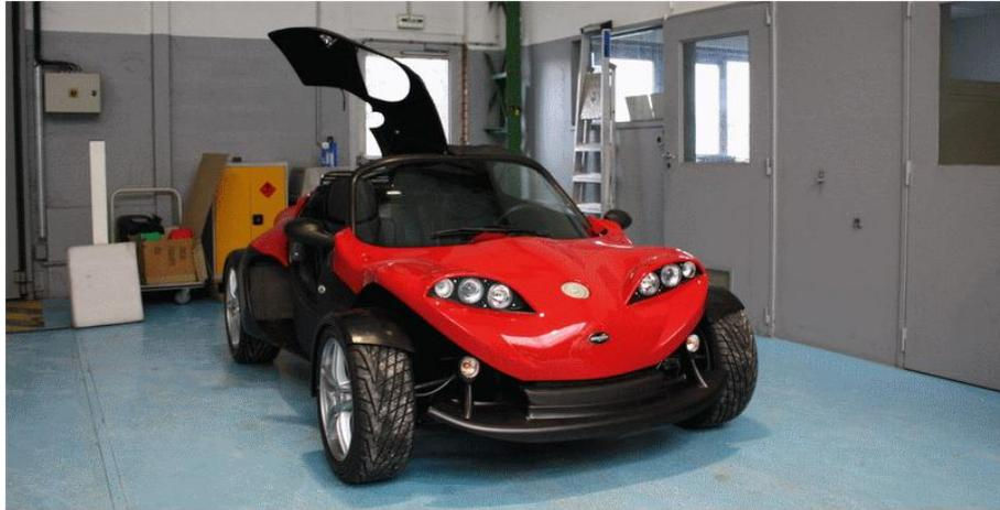
Figure 4.31: ABV Low Speed Vehicle: proprioceptive sensors and actuators have been installed. Exteroceptive sensors are now being added
