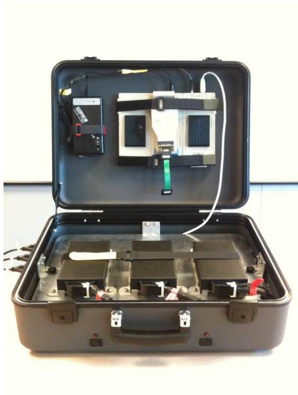
Figure 4.6: The LIVIC Legal Safety Demonstrator suit case: Continental CSC ECUs (lower half), Lauterbach Power Trace II with Nexus interface for code flashing and debugging (upper half) and connection to vehicle CAN and PC for code flashing and debugging (left side)
