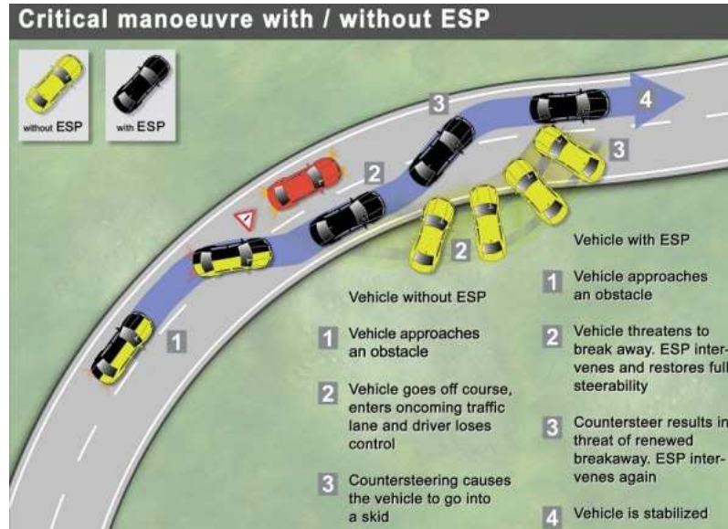
Figure 2.6: Functioning of ESC in critical situation (image from Bosch GmbH).
