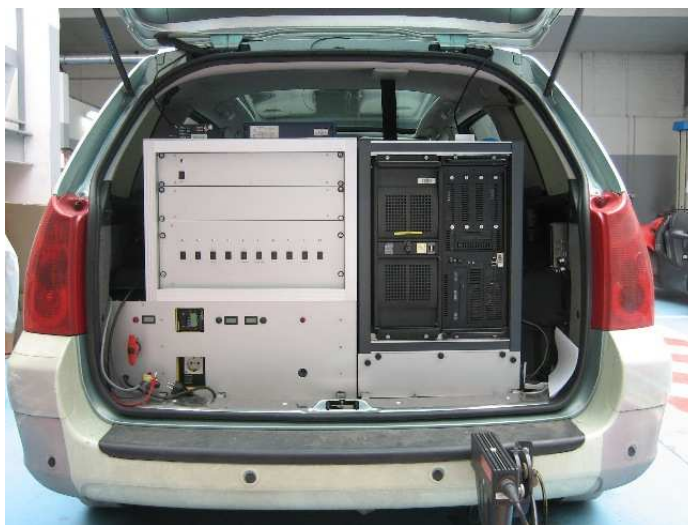
Figure 4.29: Computing units for image processing and control algorithms
