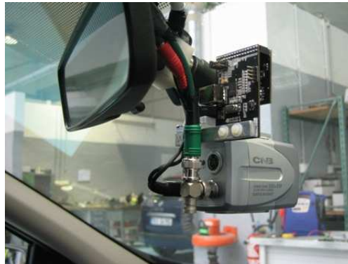
Figure 4.27: CCD video camera for frontal view
