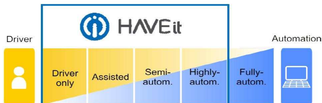
Figure 2.5: Level of automation and repartition of driving tasks in HAVEit project [HAV11].
