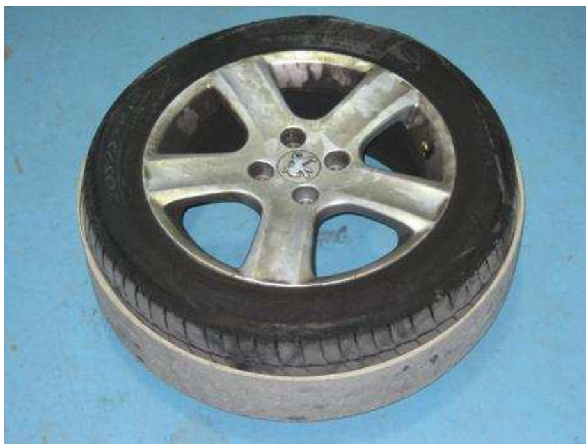
Figure 7.3: Skidconcept ring mounted on front wheel.
