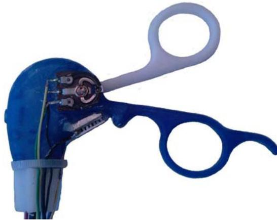
Figure 5.8: Handle sensorization for grasping angle sensing.
